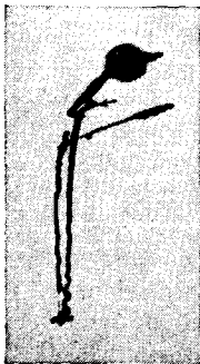
FIG. 8-39.—A (V,I) -trace from a 2J42 magnetron, showing the "attempt" to start made by the lower-voltage mode even when the tube eventually oscillates in the higher-voltage mode. (Photograph courtesy of J. V. Lebacqz.)
